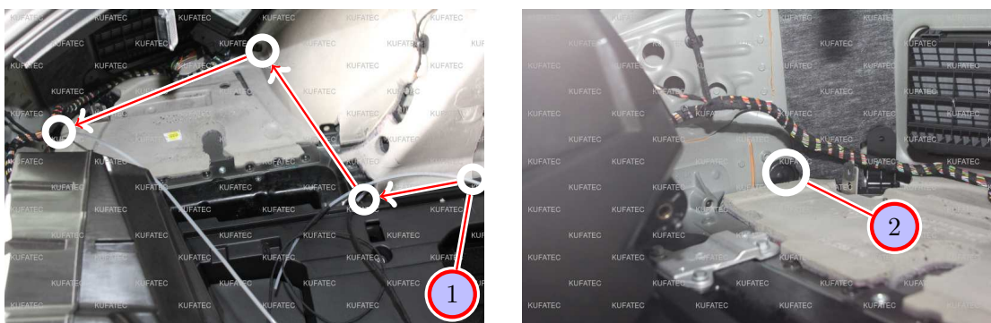
Figure 13: Cable routing to the sound generator
